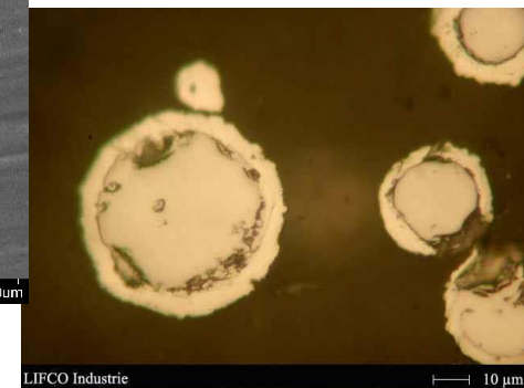
Coated spherical ceramic powder
